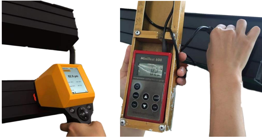
涂魔师coatmaster: 82.9 \mu m 干膜测厚仪: 82 \mu m
